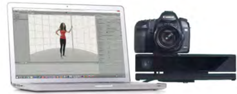
The 3-D scanning tool DepthKit combines the capabilities of DSLR camera with the Microsoft Kinect for depth sensing to create 3-D avatars of real people. PHOTO COURTESY OF DEPTHKIT
